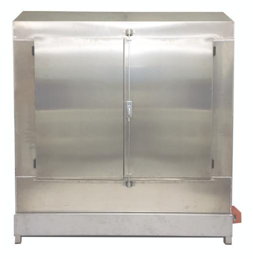
The Cromocol Tropical Chamber is designed to determine the moisture resistance of dry films and to test the ageing of adhesives and sealants under moist conditions. The test is performed under 100% relative humidity and a cycled temperature. The Tropical Chamber comes with a preprogrammed test cycle according to standard, but it also offers the possibility to set your own temperature.
