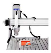
The form of the injury is to be chosen by selecting the appropriate program. The following milling programs are already preset within the delivery specification: X-shaped, L-shaped, T-shaped and diagonal shape as well as single line vertical & horizontal. By entering the sample size, the maximum injury size is calculated automatically.
