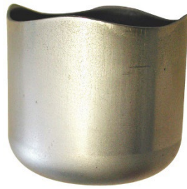
Deep Drawing Cup Test
