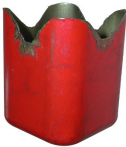
Square Deep Drawing Cup Test
