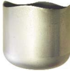
Deep Drawing Cup Test
