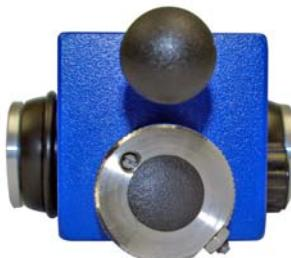
The pencil tip protrudes about 5 mm out of the holder block. Place the **TriForcePencil** carefully on the sample, set up first with the wheels and after then with the pencil tip. Lower the device slowly by index finger under the round knob of the lift arm. The hubs of the wheels are held with the thumb and forefinger and the instrument is moved over the specimen in the direction the pencil point shows at a speed of about 10 cm/s.
