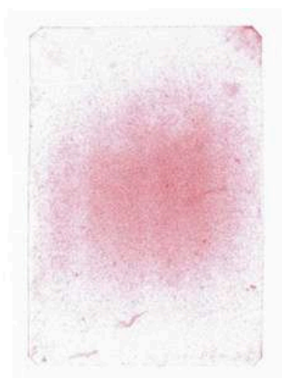
Pressure distribution on bare metallic plates
