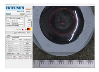
Contrast lines are now positioned by cursor, i.e. at the transition contrast from substrate to coating, as well as at the upper edge of the coating.
