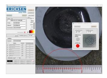
The software automatically calculates the layer thickness after entering the wedge cut angle.
